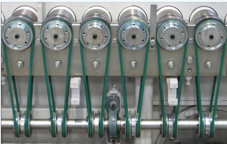
Illustration 2: Drive Belts Running On Double Pulley System
